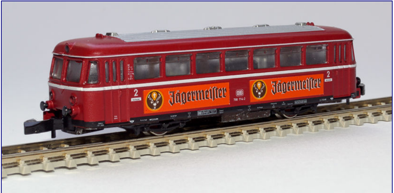
The Jägermeister rail bus (8831) was built from 1994 to 2008 with both three-pole and five-pole motors. The driving characteristics of both versions are surprisingly similar.
