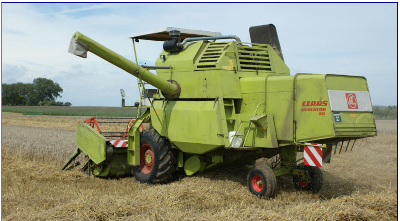
This Claas Mercator 50 (built in 1974) is the smallest model of the second-generation large combine harvester from Harsewinkel. In addition to the desire for more performance, the appearance had also become more important. The result was the side panels, accompanied by the colour seed green and a modified logo that is still common today. When this model was launched on the market in 1969, it was still called Claas Protector.
