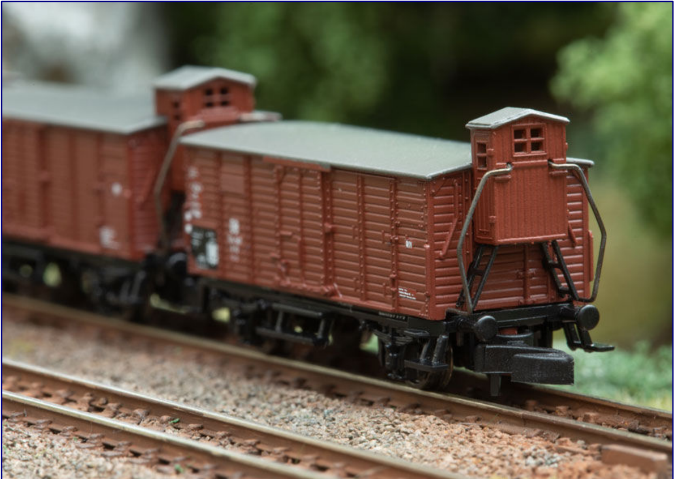
The brakeman's cab, which has been built back to the edge of the roof and is also often referred to as the "economy brakeman's cab", is a newly designed attachment part with which the five-piece G-10 freight wagon pack (86605) should appeal to its customers. Photo: Märklin
