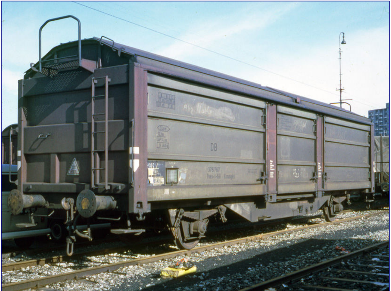
The design of this Tbes-t-68 / Klmmgks 376 767 photographed at Stuttgart's main freight terminal corresponds to the two Märklin models from set 82153. Therefore, it allows a comparison (see also photo on page 4) of some of the details: its access ladder is painted reddish brown (not black) and also the cross portal is painted in body colour (instead of roof colour as is the case with the models). Photo: Fritz Willke, © Stefan Carstens
