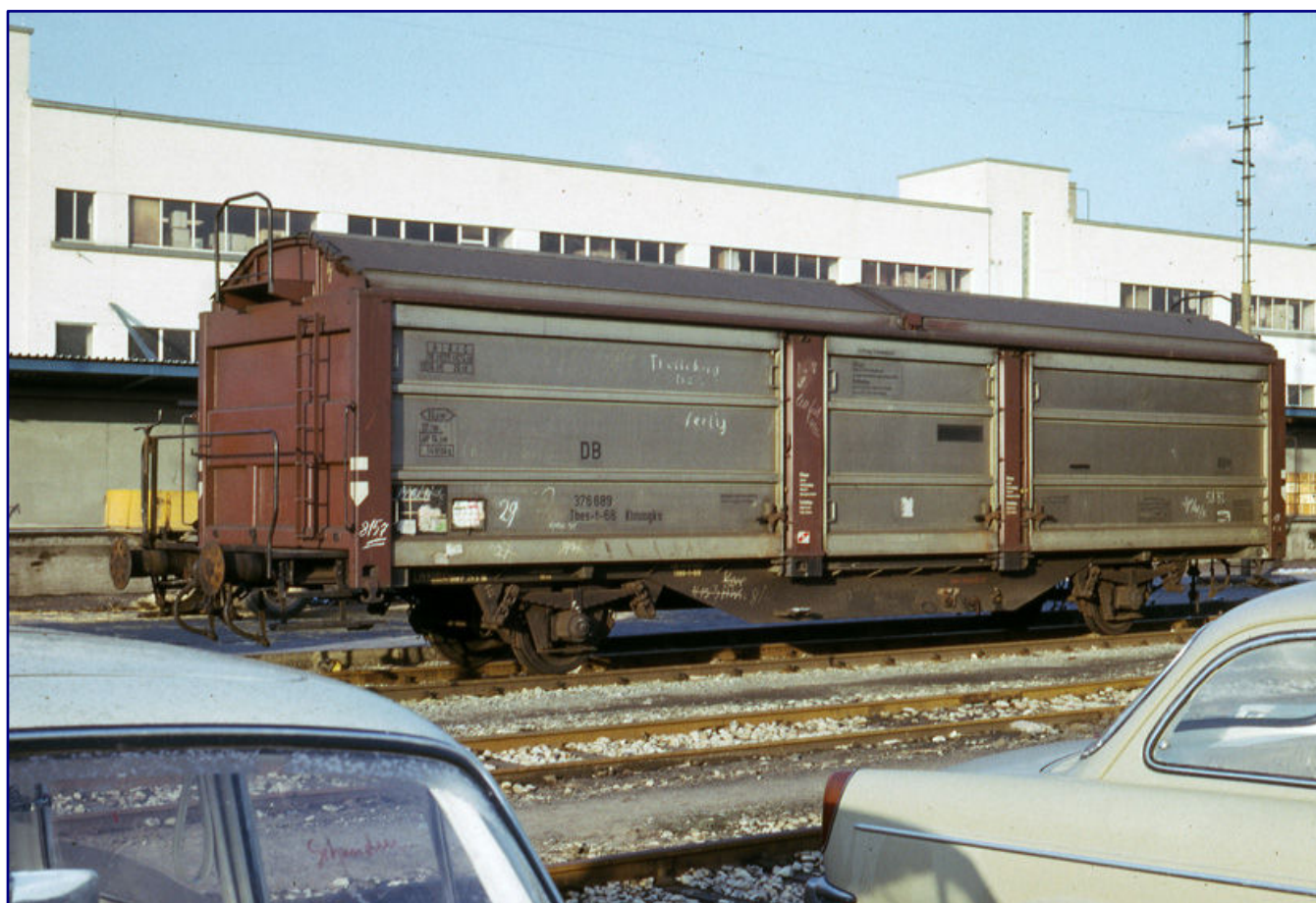
A perfect photograph of a Tbes-t-68 / Klmngks of the German Federal Railways; here, the specimen with car number 376 689. This wagon belongs the variant equipped with handbrake, and is 500 mm longer than the prototype behind Märklin's model. Nevertheless, it still serves as a valid basis for assessing the model. Photo: Fritz Willke, © Stefan Carstens
