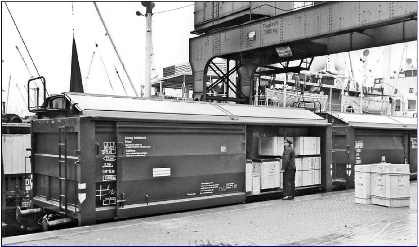
The sliding roof / sliding door cars of the later types Tbis 870 und 871 were directly derived from the Kmmgks 58 (later Tbis 858) wagon type like the one shown here at Hamburg harbour in 1957. Initially, the Kmmgks 58 and the Tbis 870 still had curved cargo doors as seen here, but later versions and all Tbis 871 were equipped with flat doors that had welded reinforcement profiles. Photo: Walter Hollnagel, Archiv Eisenbahnstiftung
