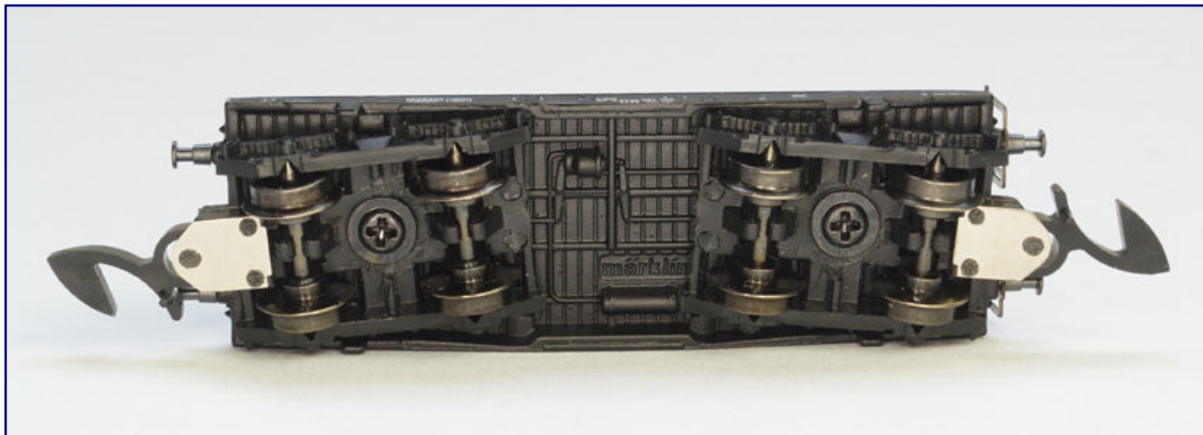
A look at the car floor bottom reveals some replicated details of the brake system and the bogies, which in this case are attached by screws.
