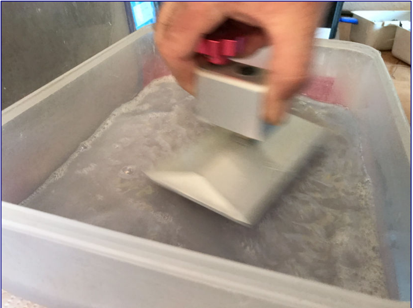
In the isopropanol bath, uncured resin is rinsed off, so that it cannot hinder the further processing of the model.
