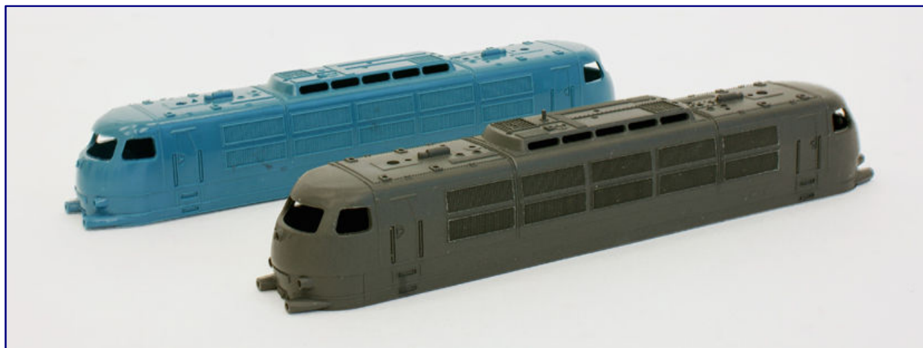
The addition of metal particles changes the colour of the material: The ABS plastic body shell is blue, whilst the metal filled plastic shell of the class 103 locomotive takes on the grey colour of the tungsten metal.
