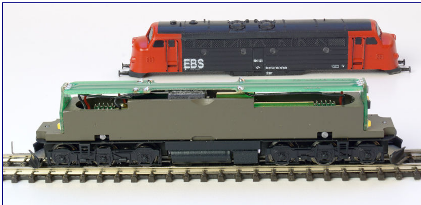
The side view allows an idea of how the three PCB elements are connected to each other. The analogue locomotive looks very tidy due to its low proportion of electronics inside.
