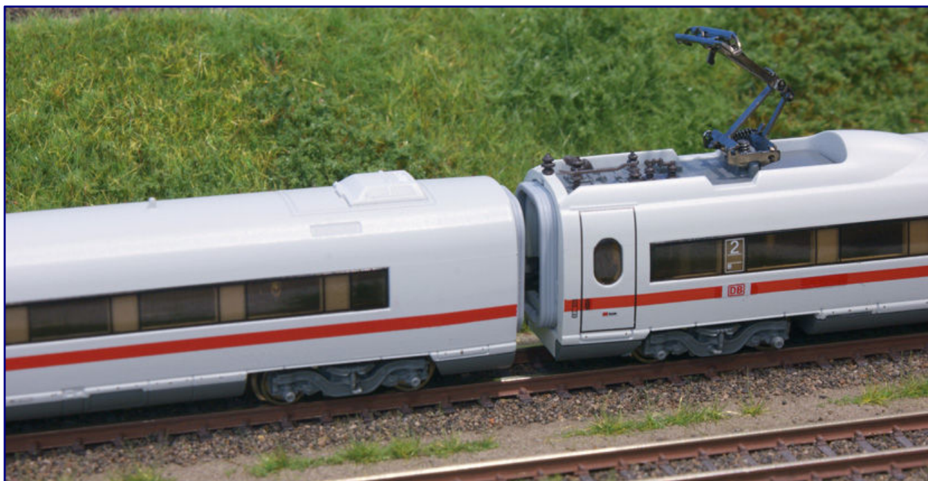
The central summer innovation at Märklin is an ICE 3 of the 406 series with newly designed intercommunications. Also the boxes of the air conditioners on the roof, which were installed later on the model, are now finally copied.
