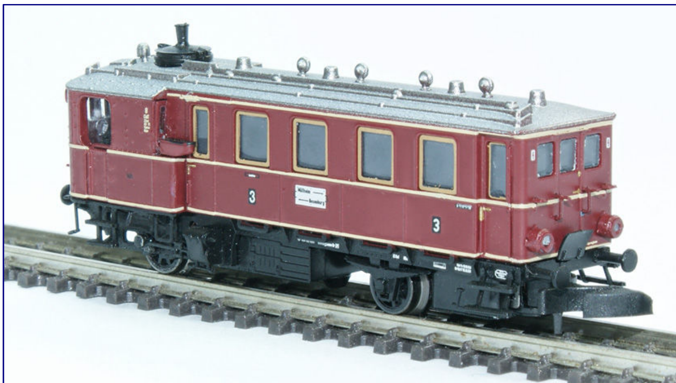
The rear end of the steam railcar has been fitted with a system coupling so that, additional wagons can be hauled on its journey.
